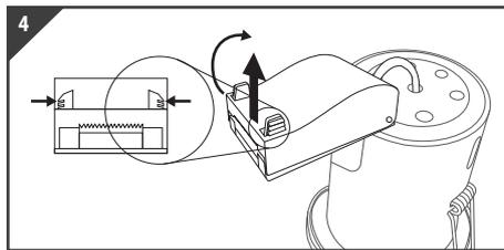
Pinch teeth together to release cable grip. Lift lid from terminal block cover.
