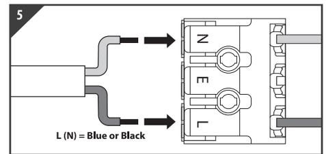
Push down the terminal, insert correct supply (as above) into terminal block and release the push fit terminal to secure. Product is Class II. E terminal for Earth provision only
