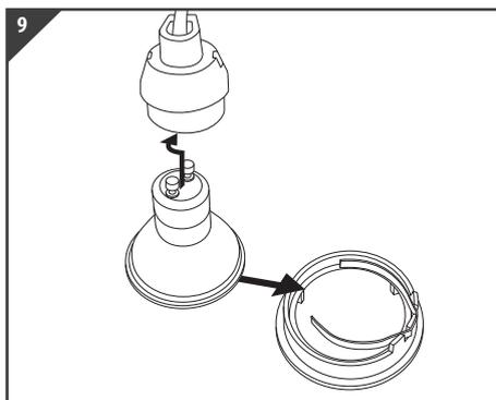
Insert correct wattage of GU10 lamp into the light socket. Slide connected GU10 into the lamp casing
