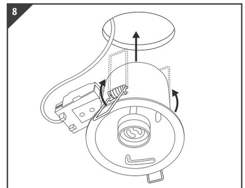
Push springs upwards against the body of the downlight and insert in the hole
