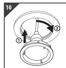
Push casing with correctly connected GU10 into the main housing. Casing will only insert when pins are aligned correctly. Twist to lock into position.
