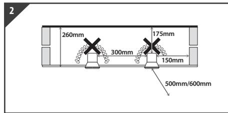
Ensure product is located in the correct location using the minimum spacings shown above. Under NO circumstances should these fittings be covered with insulation material or similar.
