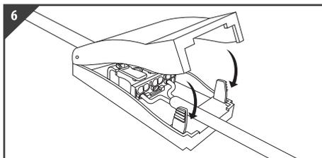
Close the cover to secure the mains cable in place
