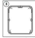
Mark the mounting surface and drill appropriate size holes for the fixings used
