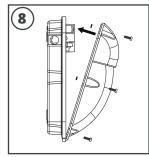
Replace diffuser cover ensuring that the rubber washer is placed over the screw thread
