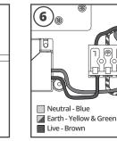
Insert correct supply (as above) into terminal block
