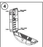
Fix the luminaire to the mounting surface using the fixings supplied
